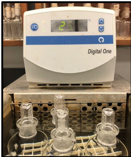
Figure 3. Water bath set to 25C showing the appropriate water level.
