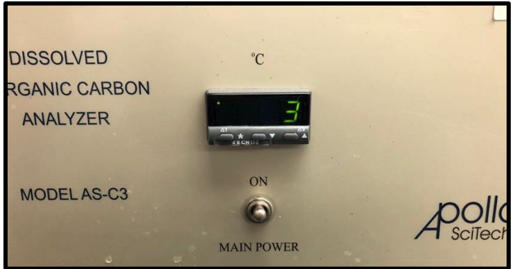
Figure 2. Temperature gauge on DIC machine. Wait until machine displays 4C and below to begin measurements.
