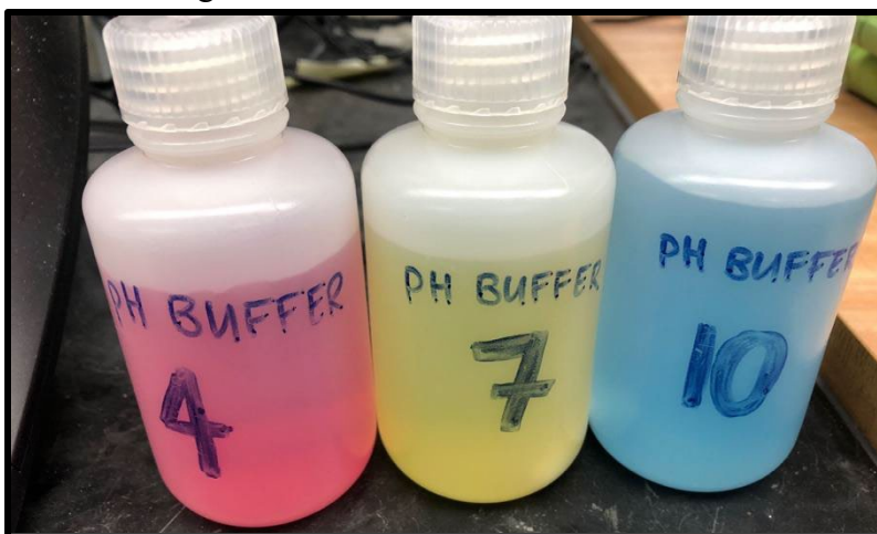
Figure 6. The three ranges of pH buffers used to calibrate the TA probe.
