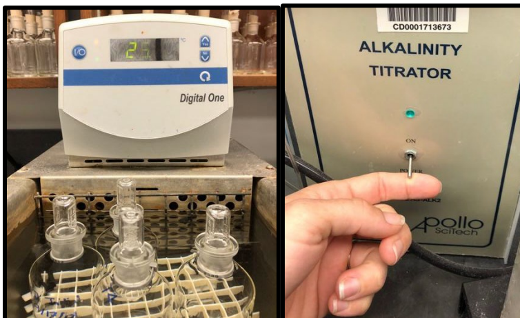
Figure 2. Photo of the water bath on the left set to 25^{\circ}\text{C} showing the appropriate water level. Photo of the TA machine on the right.
