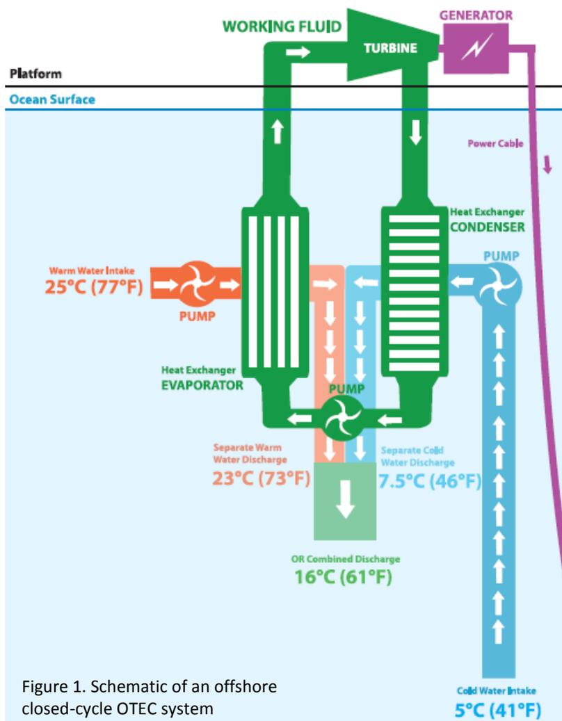
Figure 1. Schematic of an offshore closed-cycle OTEC system
