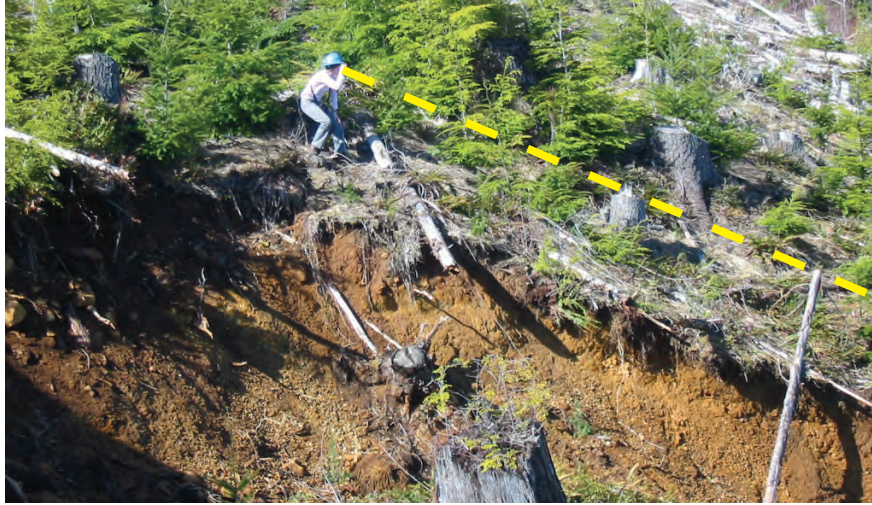
Figure 5-2: Example of measuring hillslope gradient at the failure initiation site (Photo: Julie Dieu) As shown in this photo, field crew were trained to take a hillslope gradient measurement adjacent to the landslide initiation site that best approximated the hillslope gradient at the failure site.
