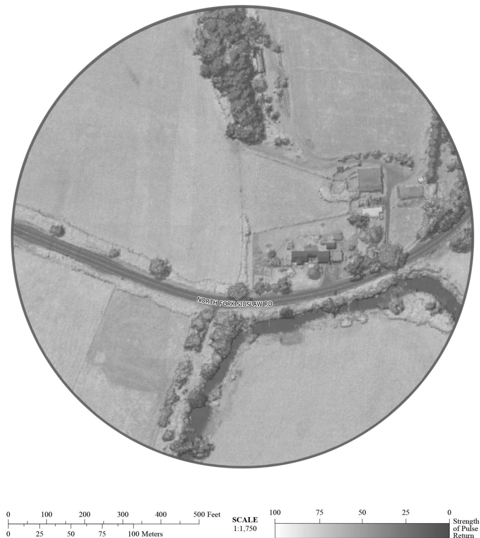
Figure 4. Example lidar-derived map displaying intensity data where white is the more reflective surface and black is the less reflective surface. Also note that the plowed agricultural field (right) and unplowed (grazing) field (left) can easily be distinguished.
