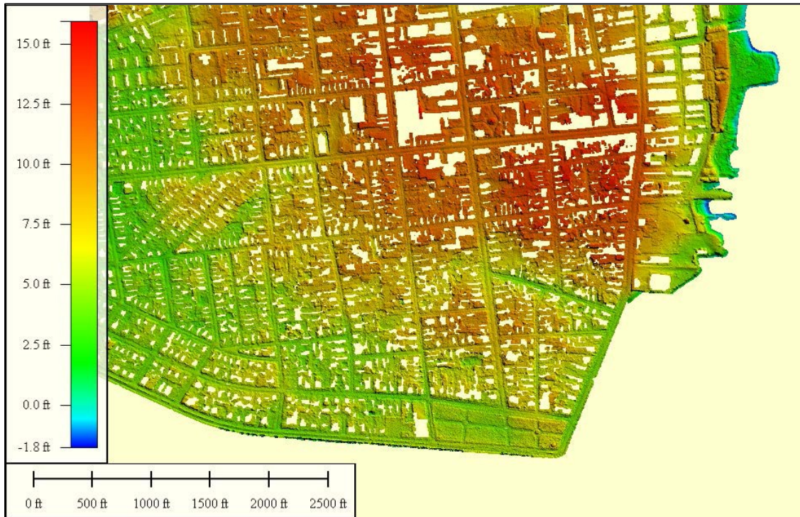
Figure 1. Charleston, South Carolina, lidar at 1-meter resolution. Note the many holes where the point spacing is below the threshold.
