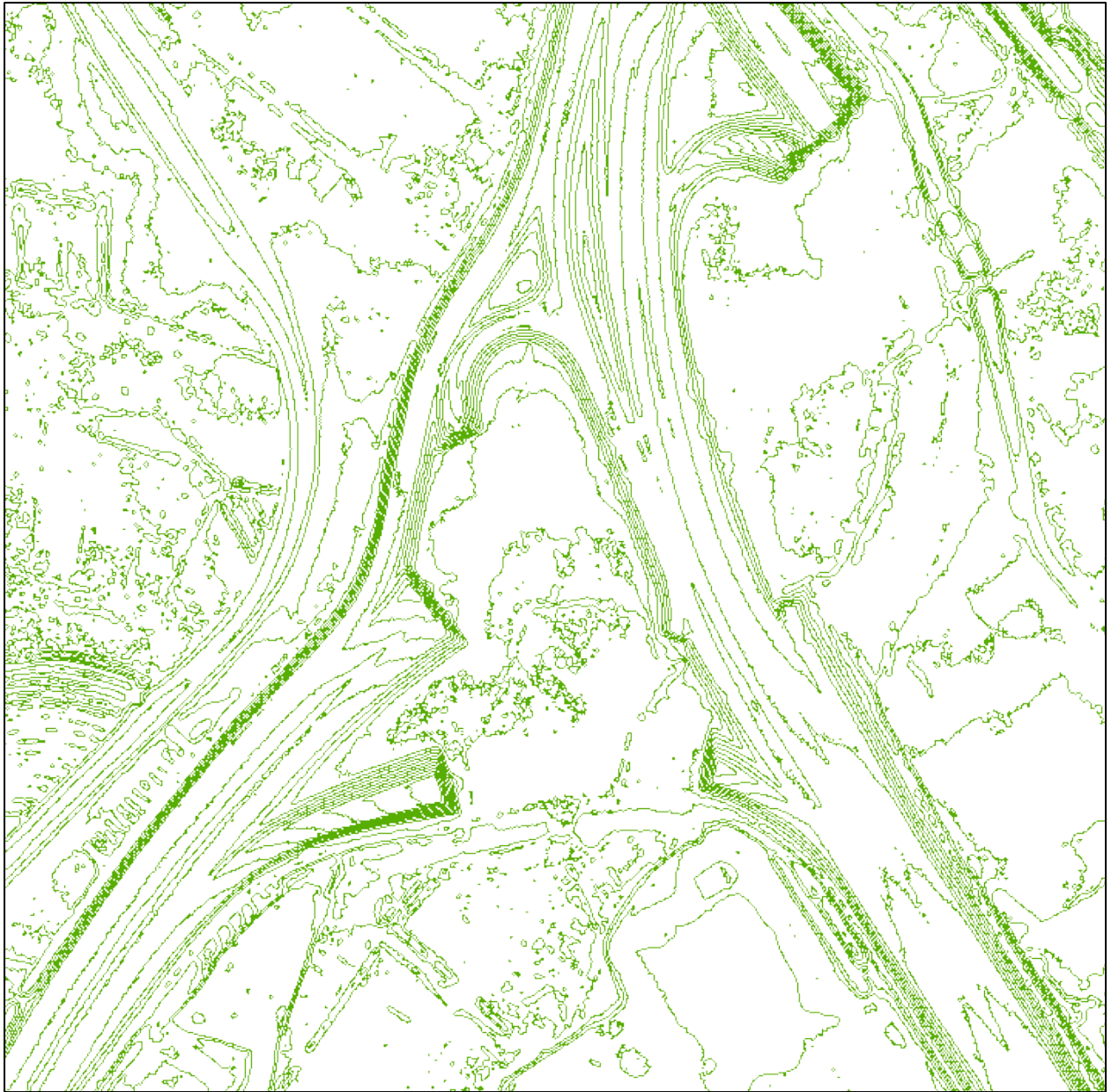
Figure 11. Two-foot contours generated on a 1-meter grid using the spline method.
