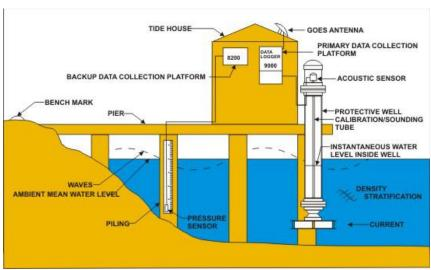
Figure 3.2. Schematic of a modern water level station
