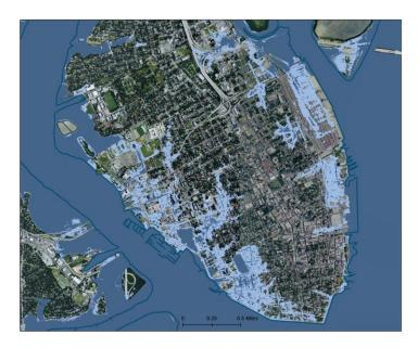
This map, based on a highly accurate lidar-derived DEM, shows areas
