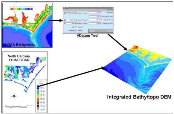
Figure 7.1. Construction of the continuous bathy/topo DEM
