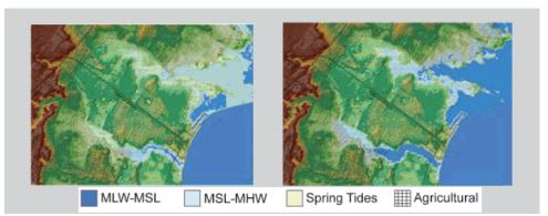
**Figure 6.3.** Johnson et al. (2006, as cited in CSP, 2009) examined SLC inundation potential for agricultural land in Worcester County, Maryland. On the left, blue areas show present-day inundation. On the right, inundation expected in 2100 using IPCC's (2001) accelerated rate of SLC is shown.
