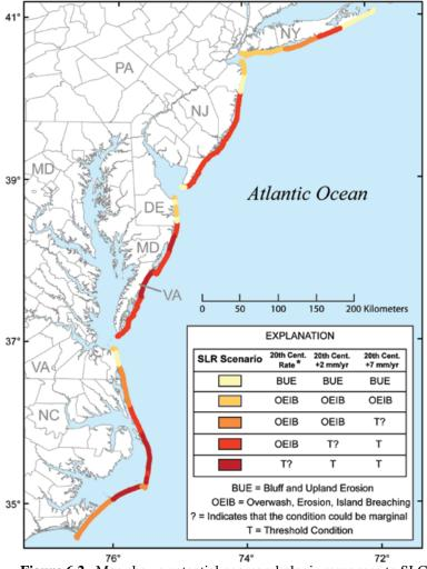
**Figure 6.2.** Map shows potential geomorphologic responses to SLC for four coastal compartments along the Mid-Atlantic region (NY, NJ, Delmarva Peninsula, VA/NC coast) (CCSP 2009). Potential responses shown in the inset table based on work by Gutierrez et al. (2007).
