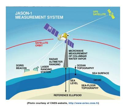
**Figure 3.5.** Schematic of a satellite altimeter configuration.
