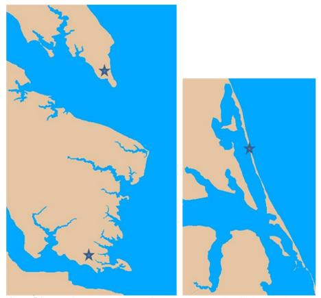
**Figure 5.9.** Locations (shown in stars) for which extrapolating tidal datums inland is more complex due to proximity to waters of different tidal regimes. The left figure shows a portion of Chesapeake Bay, and the right figure shows some of the barrier islands off North Carolina.
