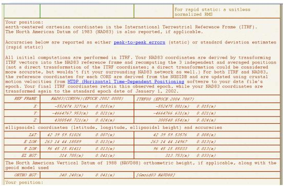
**Figure 5.3.** Sample output from OPUS, showing the *x-y-z* positional values and their associated errors.
