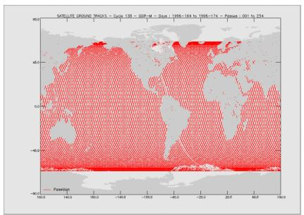
Figure 3.6. The ground track coverage for the Jason-1 satellite altimeter mission
