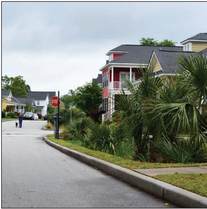
Toledo has installed bioswales similar to this South Carolina one, with vegetation and sloping sides that filter the silt and pollution from runoff.
