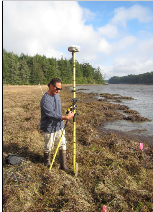
Figure 3.2: Staffer Talo Silver assisting with Real-time Kinematic Surveys at Hidden Creek Marsh, to establish elevation changes in tidal wetlands.
