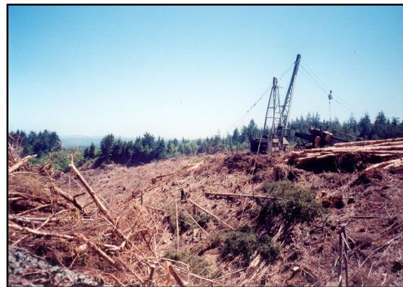
Figure 7.5: Picture of a yarder harvesting timber. Industrial timber harvest is the most common type of land use surrounding the Reserve.
