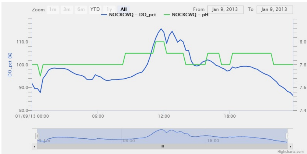
Figure 3: Day After Fish Kill Event (blue line is dissolved oxygen and green line is pH)
