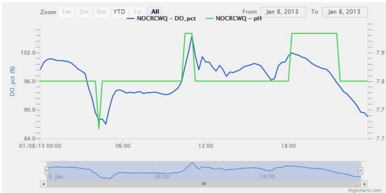
Figure 2: Day of Fish Kill Event (blue line is dissolved oxygen and green line is pH)
