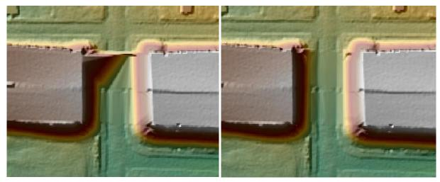
Figure 19 – Tile 470603. The left image shows a bridge saddle present in the DEM. The right image shows the DEM after bridge saddle breaklines were enforced, correcting the bridge saddle.
