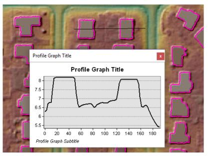
Figure 11 – Tile LID2017\_470294\_W. Impervious (pink) building outlines represent building rooftop lidar classification (class 6). Building rooftop heights are applied to the DEM with a 1-foot height buffer.
