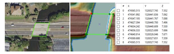
Figure 8– Tile number LID2017\_470295\_W. Orthoimagery (left) with location of bridge/overpass and corresponding overpass polyline breakline (green). DEM (right) with overpass polyline elevations representing the bridge feature. Hydrographic breaklines (blue) continue under bridge/overpass features in the DEM.
