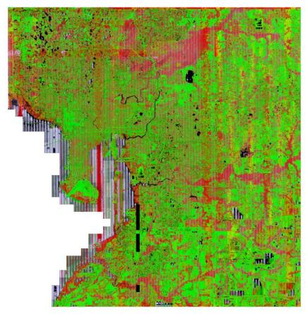
Figure 6 – Single return DZ Orthos for the Hillsborough County lidar project. Inter-swath relative accuracy passes specifications.
