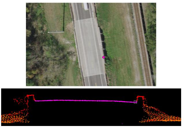
Figure 16 – Location of check point GPS098 in orthoimagery (top) and lidar (bottom). The checkpoint is located on a bridge/overpass and was not used for vertical accuracy reporting.
