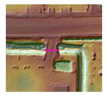
Figure 9 – Tile number LID2017\_472413\_W. The DEM shows the culvert has been left in ground and a connector (pink) was added to join the hydrographic features (orange).
